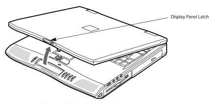
Figure 3-2 Opening the Display Panel
